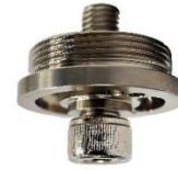
KD adapter Bolt Torque 16Nm
